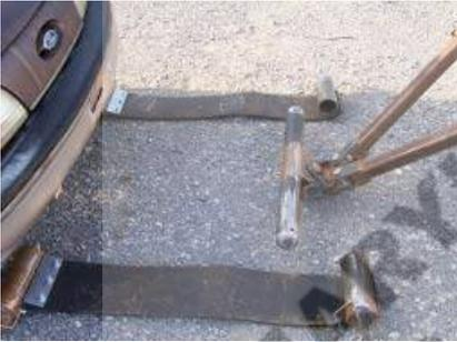
13. Remove the right hand and left hand tow sling straps for the toolbox and lay them out next to the hold back bars on their respective sides.
