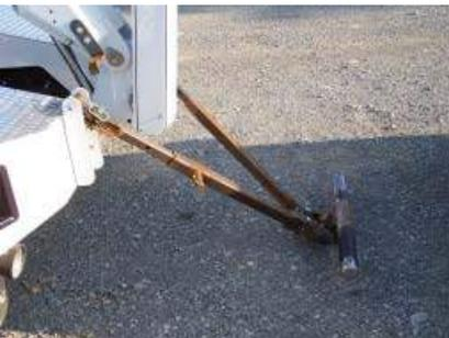
26. Open the underlift lockout valve, then partially lower the boom and underlift for easy access.
