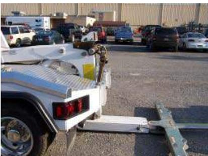
31. Fold the underlift to the ground. Lift the lower anchor assembly into the cradle bracket on the knee boom.
