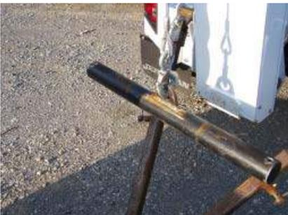
15. Remove the upper anchor assembly from the toolbox and install the hook on the winch wire rope/cable through the lug on the crossbar.
