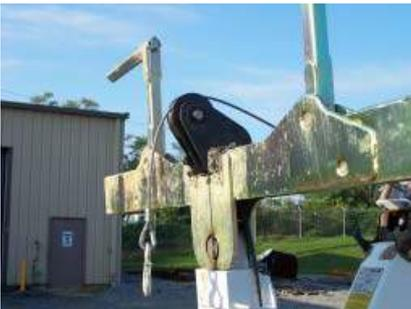
7. Route the winch wire rope/cable over the sheave and install the guide pin in the outer most hole to retain the cable.
