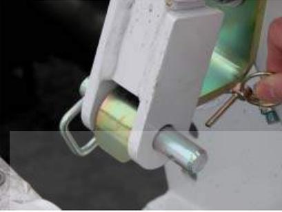
32. Connect the hold back bars to the tow sling storage bracket using the pins that you removed earlier.
