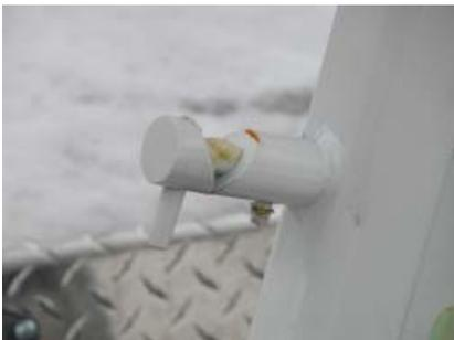
11. Position the lower anchor assembly on the ground behind the truck and turn the "CAM" handles on the back bars 90°.
