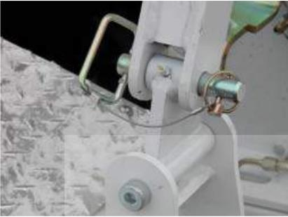
12. Connect the hold back bars to the tow sling lugs using the pins that you removed earlier.
