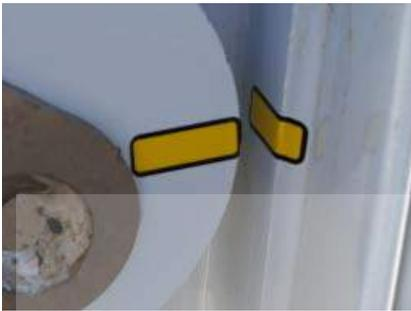
8. Fold the underlift up until the alignment indicators on the underlift and on the knee boom match up.
