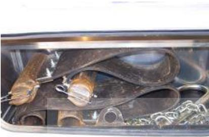
27. Disassemble the tow sling by removing the strap assemblies and the upper anchor cross bar and stowing them in the toolbox.
